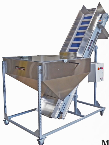
HD-Series with 15 Cubic Foot Hopper
