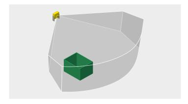
The radar technology reacts sensitively to movements. However, static objects in the monitored area do not cause the safety signal to switch off.
