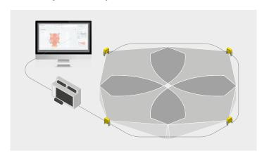
To guard large areas, up to 6 sensors can be combined in one application using a control unit. The system parameters are set using the easy-to-use confi guration software.
