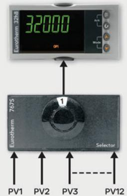
When combined with the model 767S selector switch up to twelve thermocouples or 2-wire signals, and six Pt100 signals can be viewed using one indicator. Selection is made via a front panel rotary switch which includes clear indication of the channel selected.
