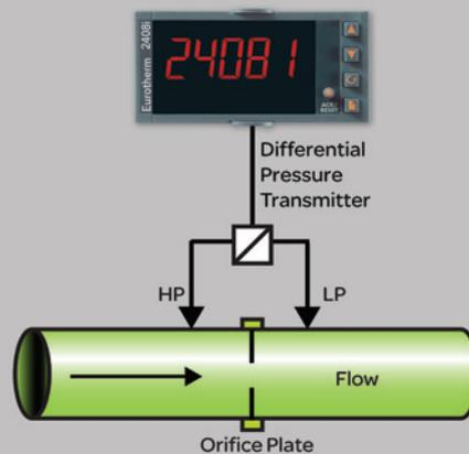
Measurement display using square root extraction to display directly the flow from differential pressure measurements using, for example, an Orifice or Venturi meter.
