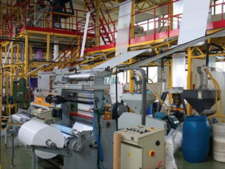
**Plastics extrusion** is a process in which raw plastic is melted and formed into a continuous profile, producing items such as pipe/tubing, window frames, plastic tape and wire insulation. To ensure they were working at maximum efficiency and operator safety is maintained at the highest levels, our customer needed to upgrade a number of extruders in his factory
